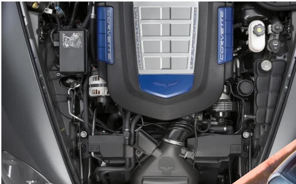
an overhead view of a 6.2-liter supercharged LS9 V-8 in Chevrolet Corvette C6 ZR-1
